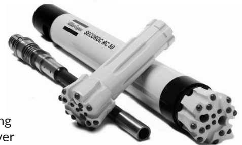
Photo 3. A down-the-hole hammer and its associated bit. (Atlas Copco - Secoroc/Epiroc) (Note: in Wisconsin these bits must be a minimum of 6-inches in diameter to construct the lower open drillhole.)
