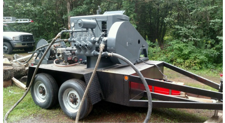
Photo 5. A hydrofracturing pump and its associated equipment. (Courtesy Dean Funk, Rhinelander Well Drilling)
